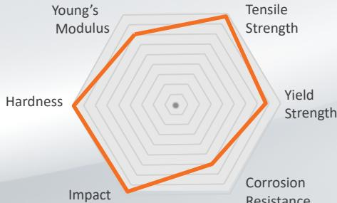
This unique austenitic stainless steel has superior strength and corrosion resistance in comparison with conventional stainless steels such as 317L, 316L, 304L and 321, whilst it still is available at a competitive price. D-50 builds on the UNS S20910 XM-19 material specification, offering consistent superior mechanical strength.
